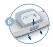
Press battery latch down and slide charger off battery.
